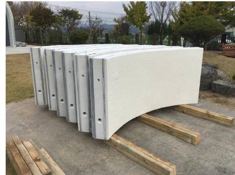
**Fig. 7.** Spraying the one-component waterproofing membrane on the segment specimens
