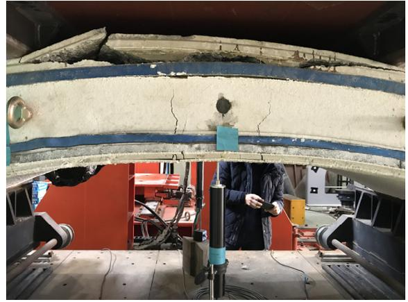
(b) Center line view after failure
