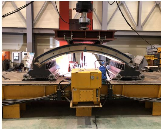
Fig. 9. Panoramic view of a full-scale bending test on a segment specimen
