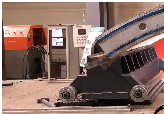
Fig. 10. Roller base for a full-scale bending test
