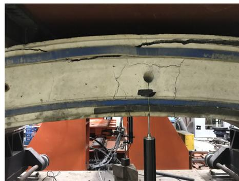
(b) Center line view after failure
