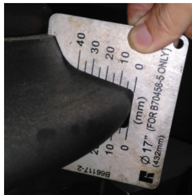
Fig. 2. Manual measurement of disc cutter wear(Liu et al., 2017)
